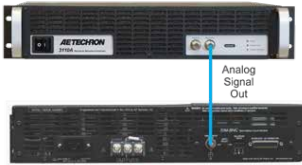
Figure 2.2 – Connecting an amplifier to the 3110A
