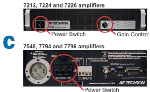
Figure 2.5 – Amplifier gain control and power switch.
